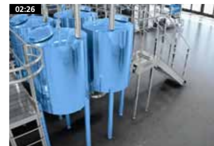
02:26 Hot water sterilization system - GEA Liquid Processing design
