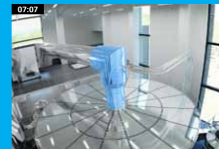
07:07 Efficient drying air inlet by use of DDD air dispenser - GEA Niro design
