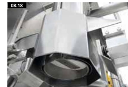
Bottom-up filling" to reduce dust emissions and product loss - GEA Avapac design
