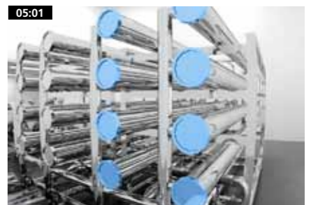
8" pressure vessels fitted with spiral-wound membranes - GEA Filtration design
