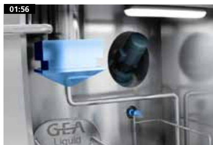
01:54 Silo tank ventilation funnel - GEA Liquid Processing design
