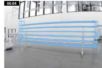
HIPEX unit for pre-heating of spray dryer feed before atomization
