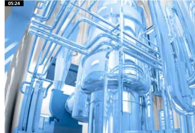
Legal pasteurization integrated in the evaporator - GEA Process Engineering France
