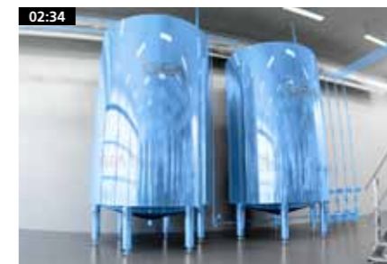
02:34 Double-jacketed stainless steel tanks and piping for CIP detergents - GEA Liquid Processing design
