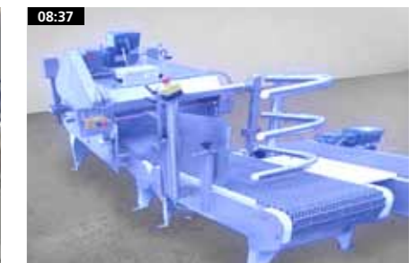
Automatic bag handling and conditioning - GEA Avapac design
