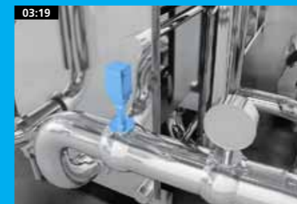
Pressure surveillance on all PHE's on all sections - GEA Liquid Processing design.
