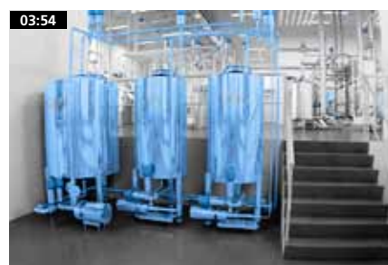
Vitamin dosing system - GEA Liquid Processing
