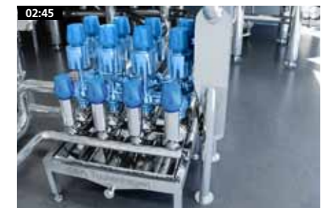
02:45 Double-seal valves on CIP lines - GEA Tuchenhagen design
