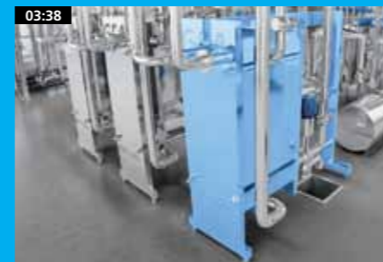
Double section cream chiller - GEA Ecoflex
